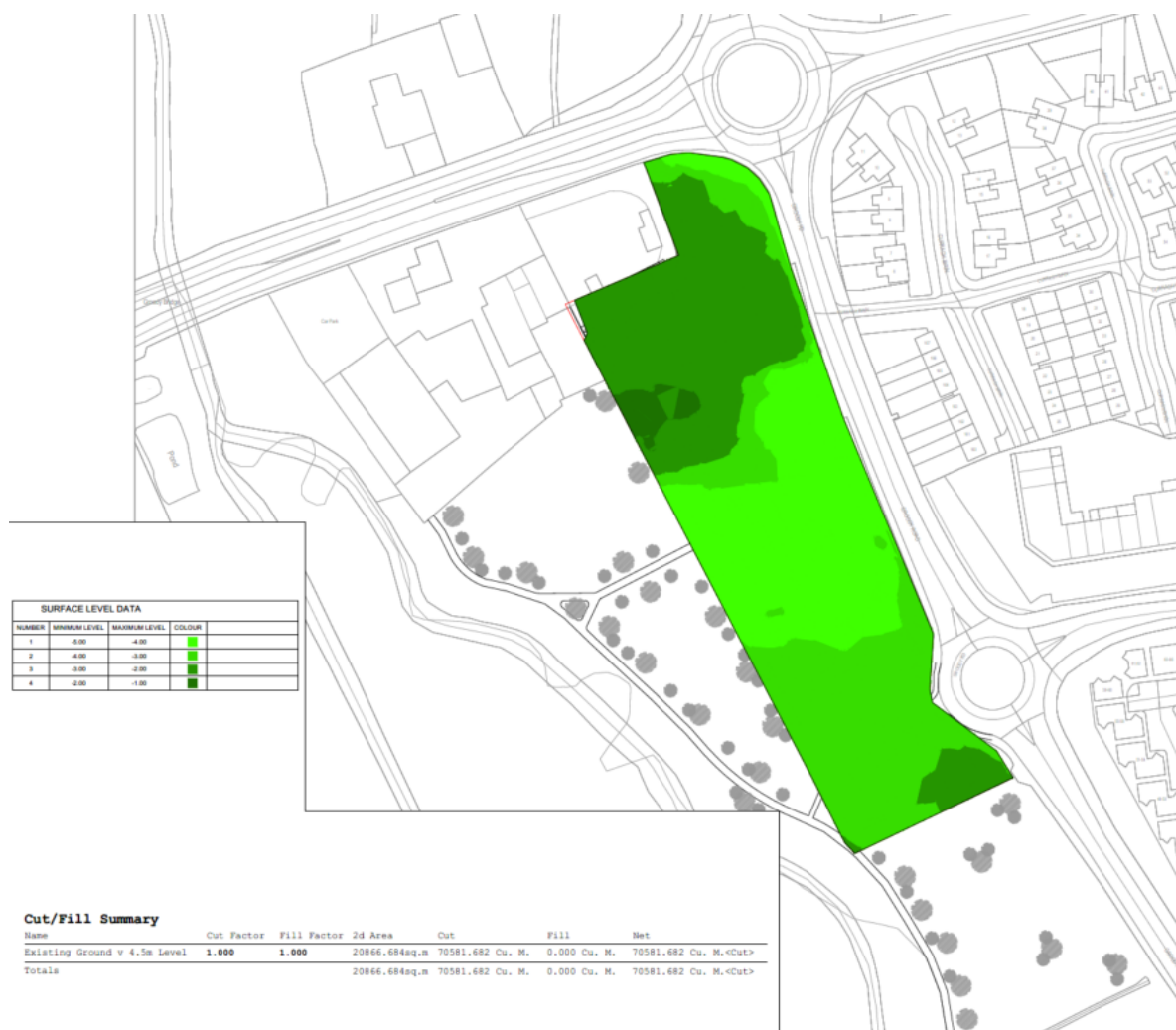
Figure 5 - Estimate of Filled Ground
